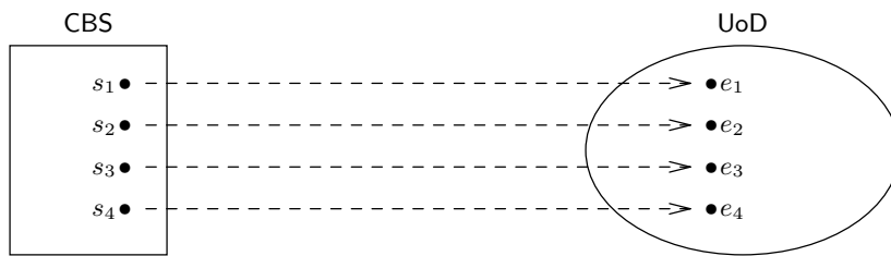
Figure 11.4: Each UoD entity is represented by a surrogate in the system. The dashed arrows indicate that each surrogate represents a UoD entity.
